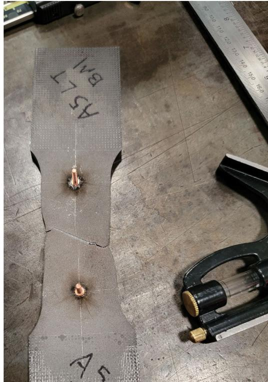
Figure 9 - Post-test photo of a tensile specimen.
