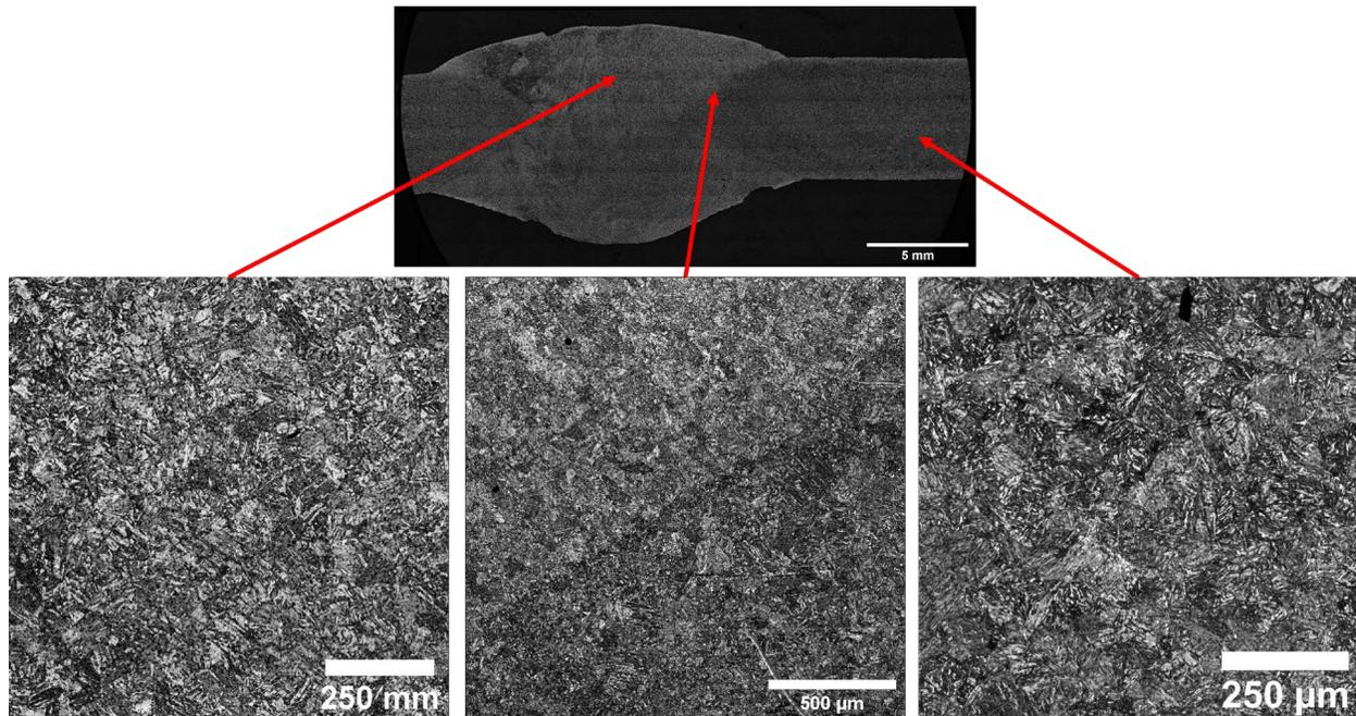
Figure 16 – Optical image of seam weld illustrating the consistent grain size between the weld metal, heat affected zone, and base metal (AM2 ATT).
