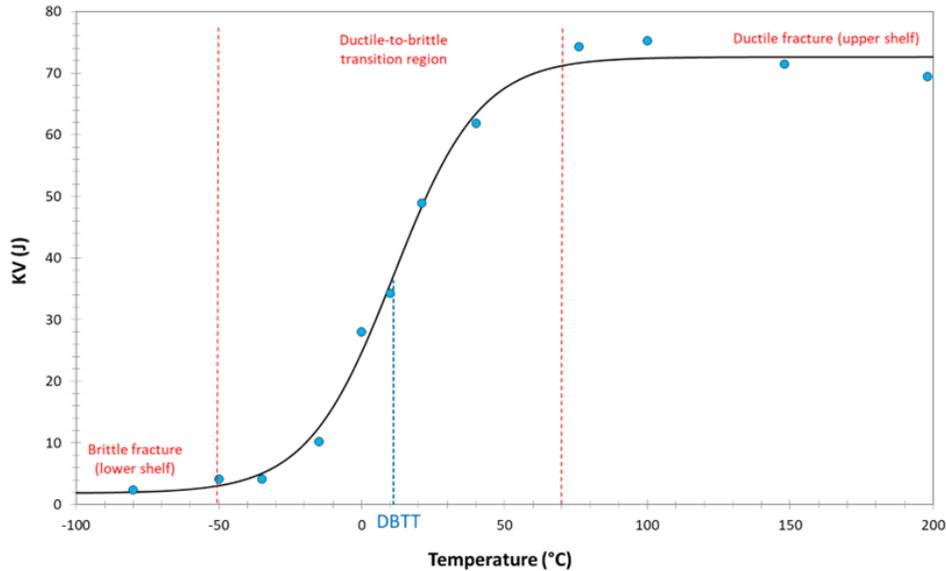
Figure 13 - Example of absorbed energy transition curve for a low-strength steel.
