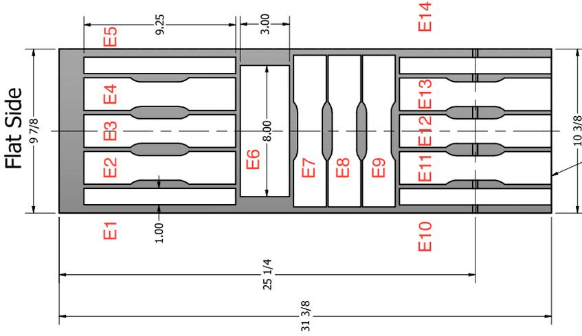
Specimens with welds must be aligned axially and centrally with the weld center line.
