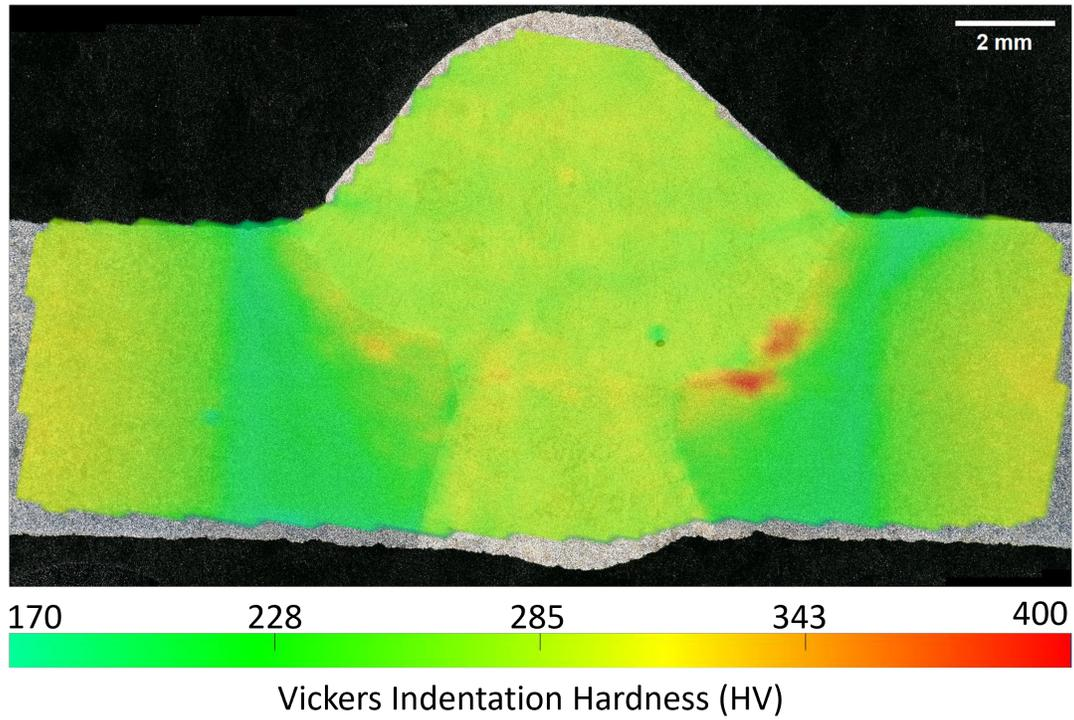
Figure 30 – Vickers indentation hardness map of girth weld (EM1 ATT)
