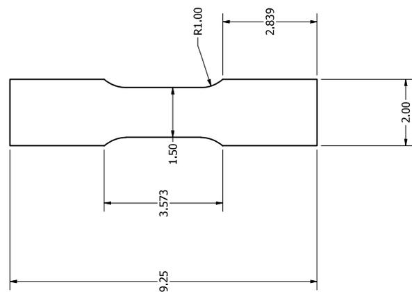
It is very possible that there isn't enough material at this end to actually cut. The important setup requirement is that the weld center line is in the middle of the specimens.
