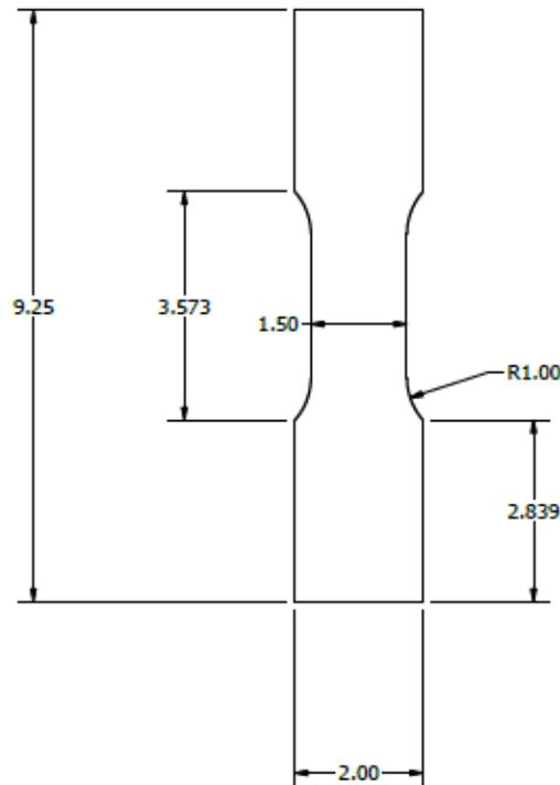
Figure 7 - Nominal shape and dimensions of full-wall-thickness tensile specimens. All dimensions are in inches.
