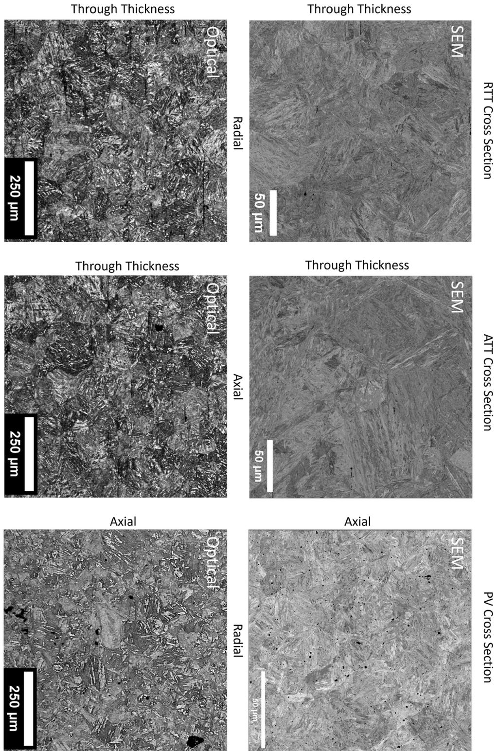
Figure 14 – Scanning electron microscope backscatter images (EM3 RTT, EM3 ATT, EM3 PV) and optical bright field images (AM1 RTT, AM1 ATT, AM1 PV) demonstrating the typical microstructure of the pipeline base metal.
