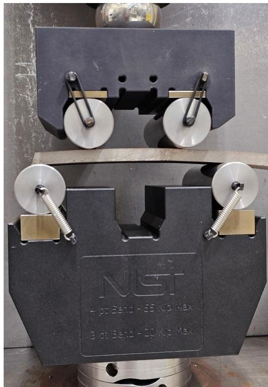
**Figure 8 - Flattening fixture used for transverse tensile specimens. Four-point bend arrangement with a lower span of 4 in and upper span of 2 in.**
