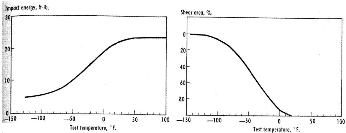
Figure 2 - Charpy test data (absorbed energy on the left and shear fracture on the right) reported by R. S. Ryan (1965).
