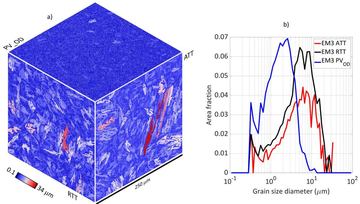
**Figure 23 - Single-tile small-area EBSD maps were recorded from all three orthogonal views (ATT, RTT, and PV<sub>outer diameter</sub>) of the base metal at location EM3. The a) grain size diameter maps and b) grain size diameter histograms provide quantitative differences between the microstructure at the surface of the pipe (PV<sub>outer diameter</sub>) and the interior microstructure.**
