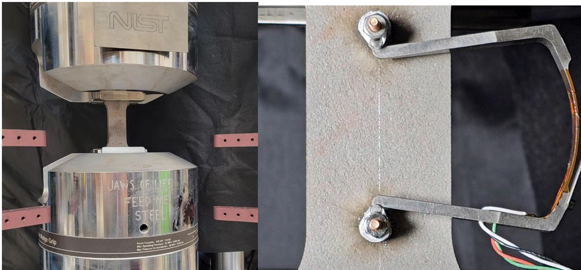
Figure 10 - Full wall thickness tensile specimens were tested in a servo-hydraulic universal test frame and were gripped in hydraulic grips (left). A close-up view of the gage section of the specimen on the ID side shows how the extensometer is attached to the specimen prior to testing (right).
