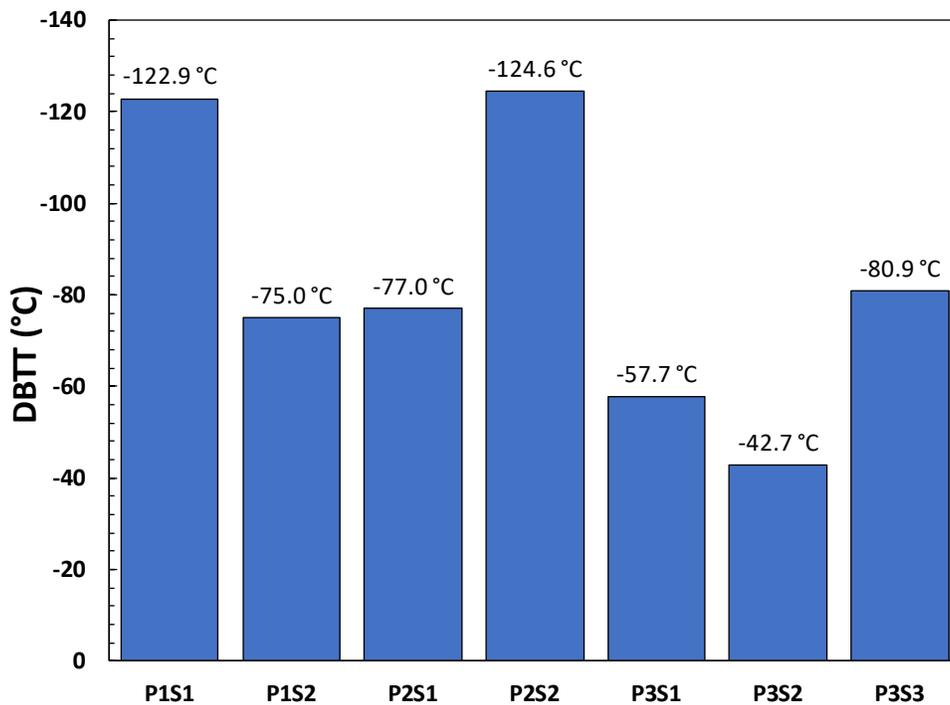
Figure 25 - Comparison between DBTT values calculated for the base metals of the different pipes and sections in L orientation. Note: the toughest conditions correspond to the tallest bars (P1S1 and P2S2).
