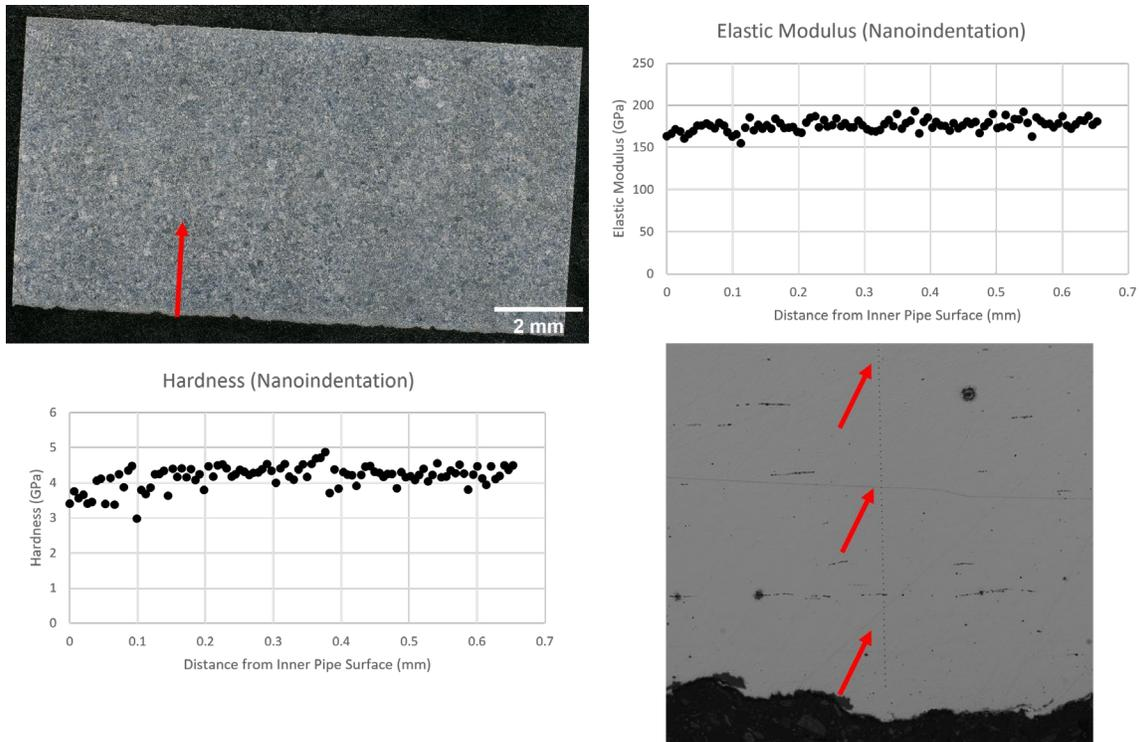
Figure 28 - Nano-indentation hardness and elastic modulus originating from the inner surface of the pipe (specimen XMX RTT).
