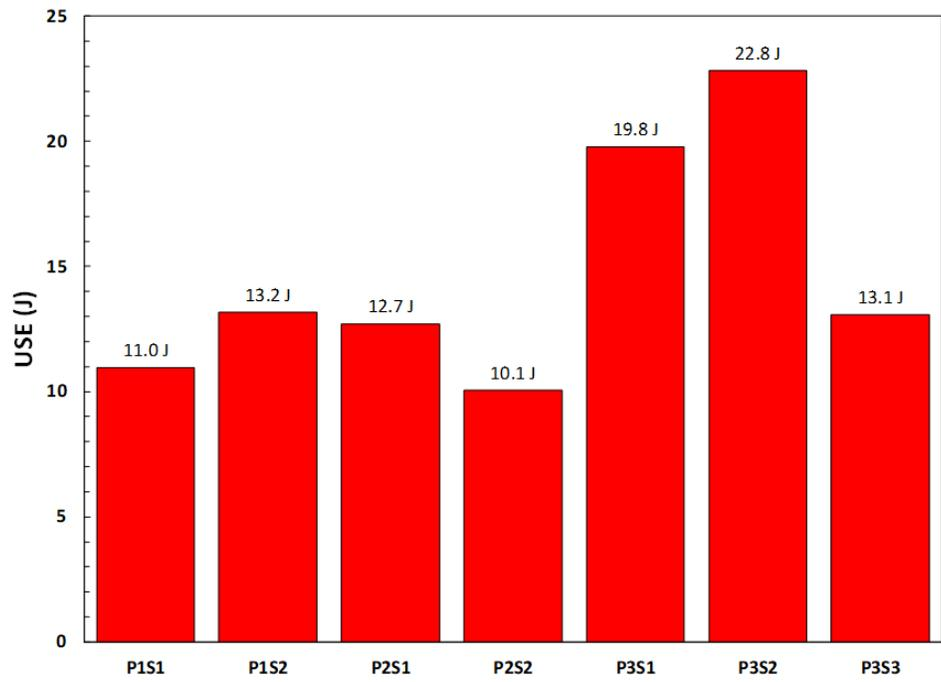
Figure 26 - Comparison between USE values calculated for the base metals of the different pipes and sections in L orientation.
