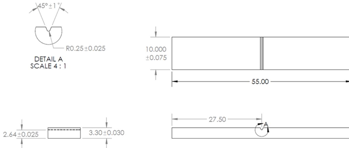
**Figure 5 – Third-size Charpy specimens used in this investigation.**
