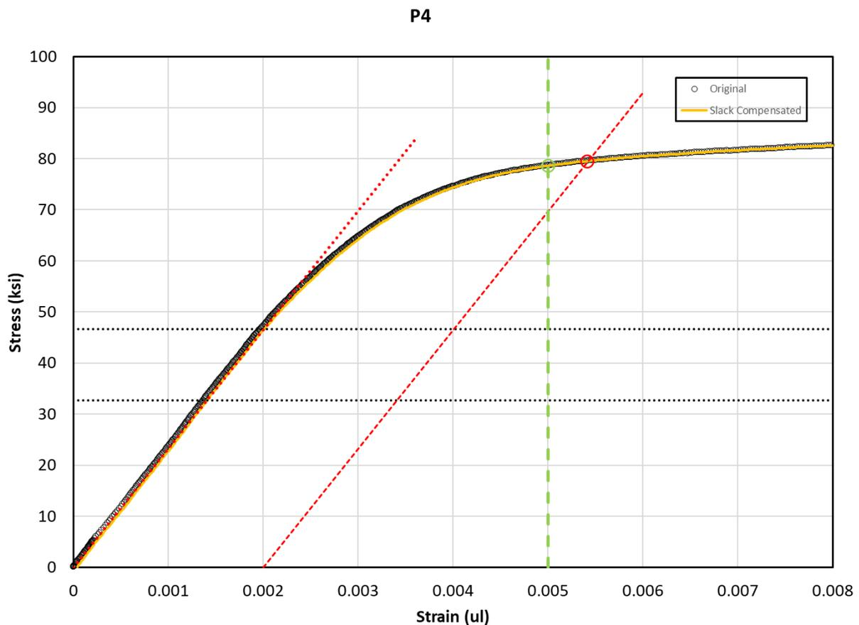
**Figure 11 - Stress-strain curve of specimen P4 (from P3S2), illustrating the Slack Plot used in the data analysis spreadsheet. The slack compensation for this specimen was minimal, resulting in a uniform elongation difference of 0.003 %.**
