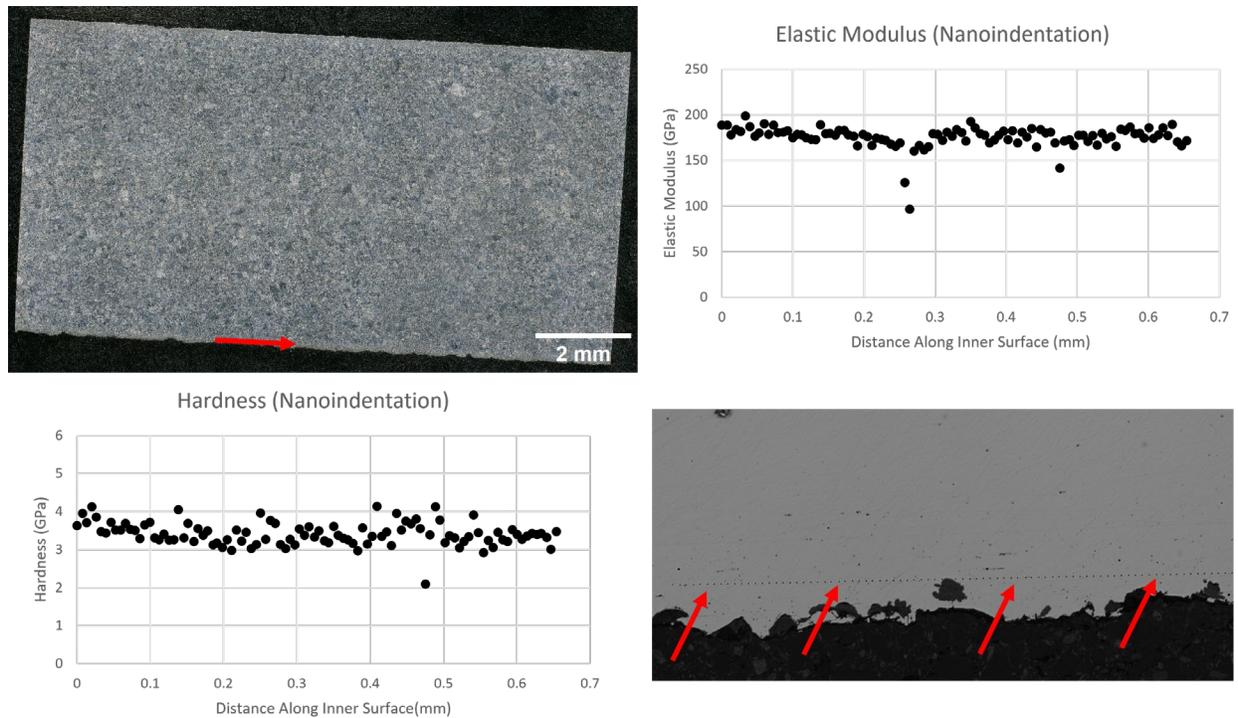
Figure 29 - Nano-indentation hardness and elastic modulus tracing the inner surface of a pipe section (specimen XMX RTT).
