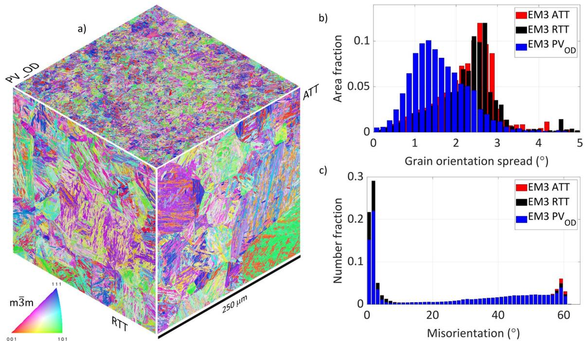
**Figure 22 - Single-tile small-area EBSD maps were recorded from all three orthogonal views (ATT, RTT, and PV\_outer diameter) of the base metal at location EM3. The a) inverse pole figure maps, b) grain orientation spread, and c) misorientation histograms provide quantitative differences between the microstructure at the surface of the pipe (PV\_outer diameter) and the interior microstructure.**
