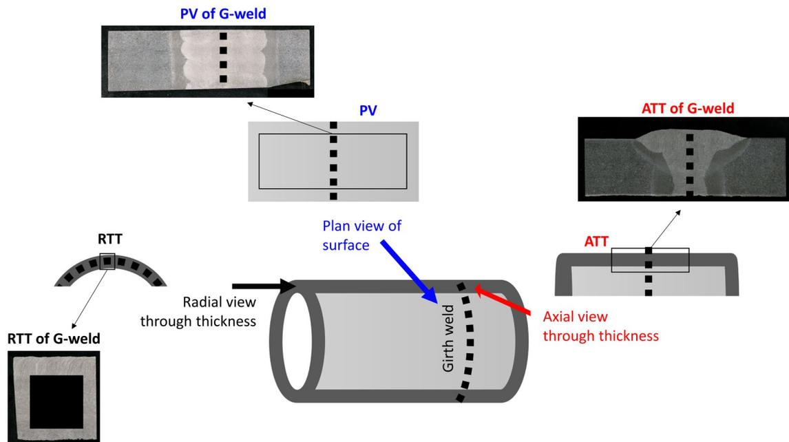
Figure 17 - Schematic of the three orthogonal views (PV, RTT, and ATT) characterized with scanning electron microscopy.
