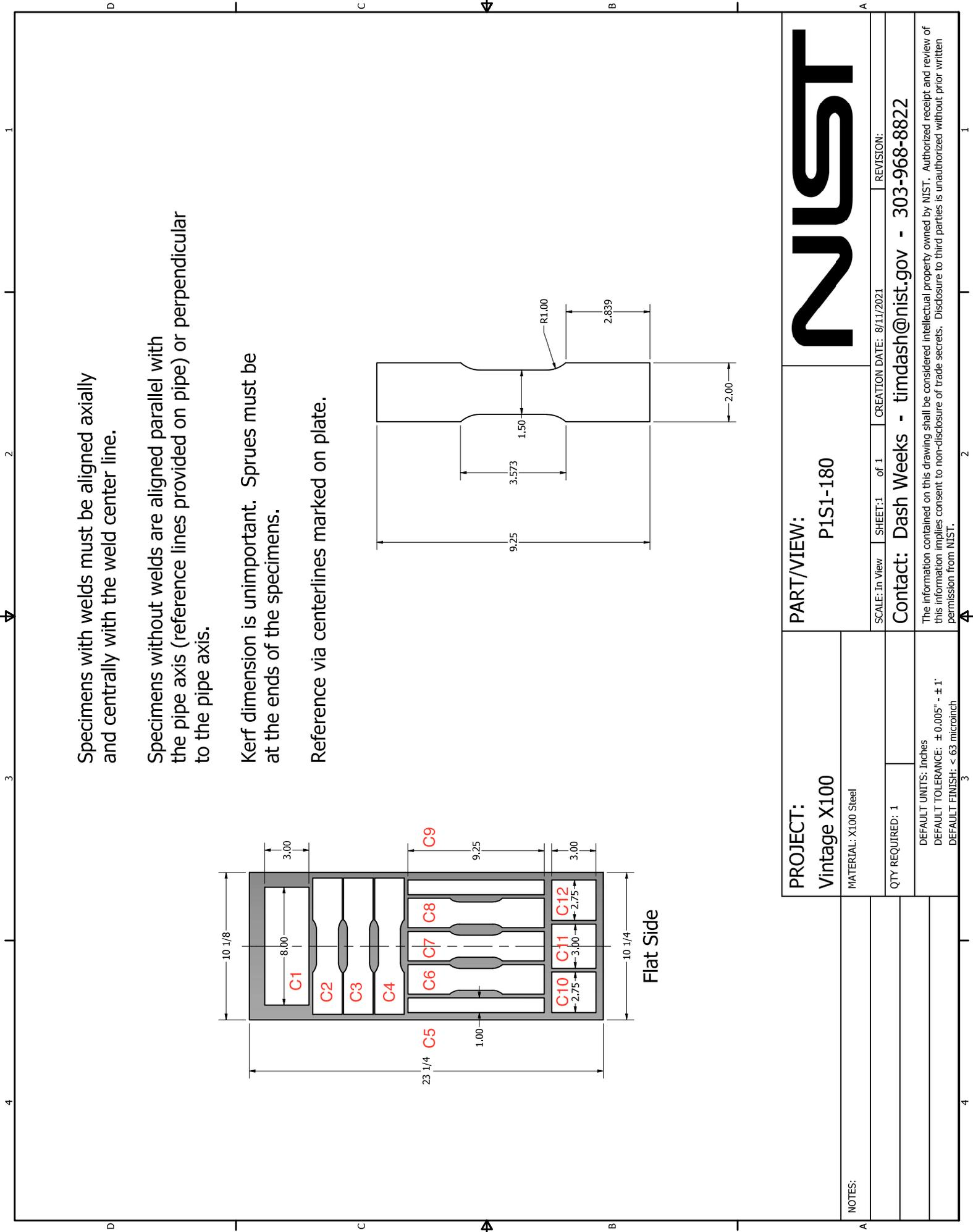
Specimens with welds must be aligned axially and centrally with the weld center line.
