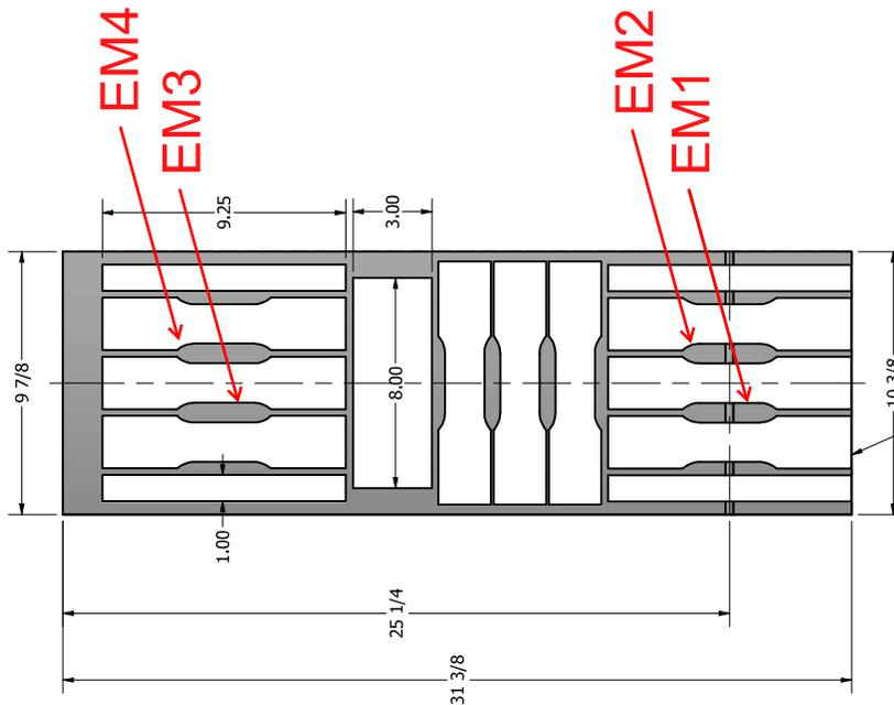
Specimens with welds must be aligned axially and centrally with the weld center line.
