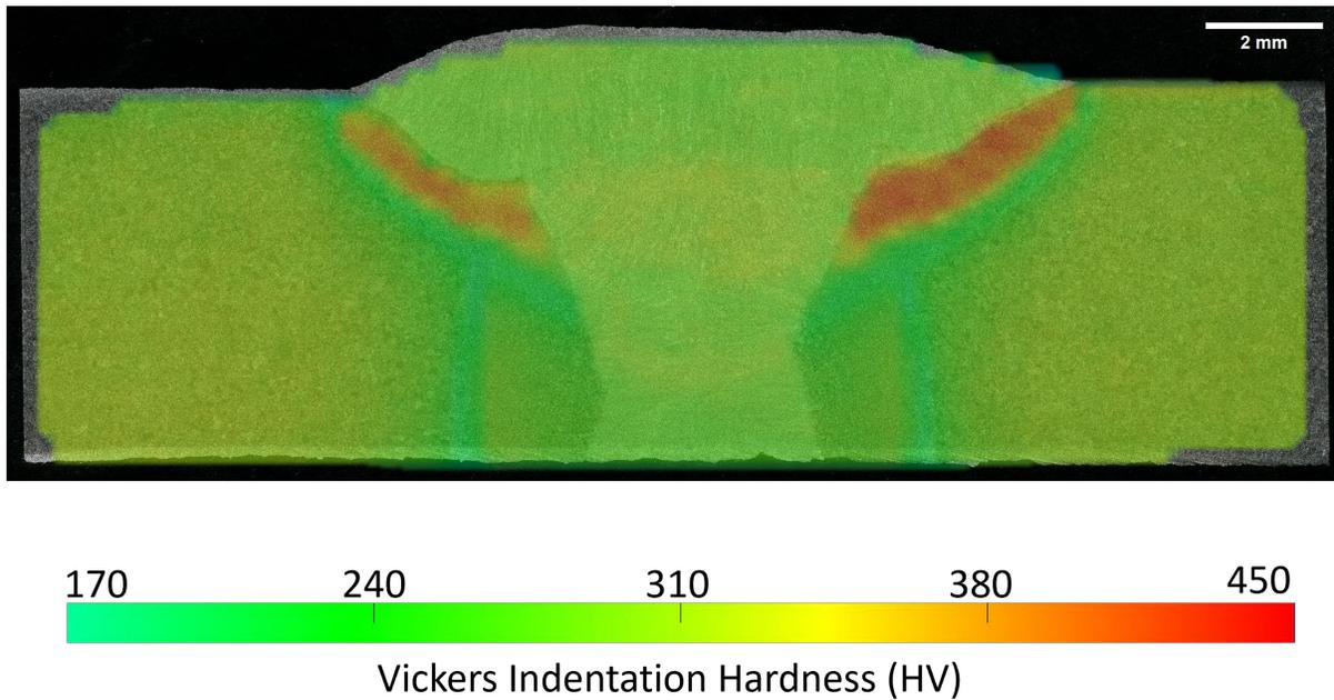
Figure 31 – Vickers indentation hardness map of girth weld (KM2 ATT)
