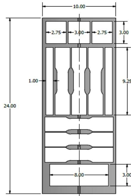
**Figure 4 - Example of a specimen sectioning plan sent to the waterjet vendor. This plan is for section P1S1, all dimensions are in inches, more detail may be found in Appendix C. Specimen blanks shown are used for CVN, tensile, SE(B) and SE(T) tests. Samplings for microstructure, chemistry and micro-hardness maps are taken from remaining sprue material.**
