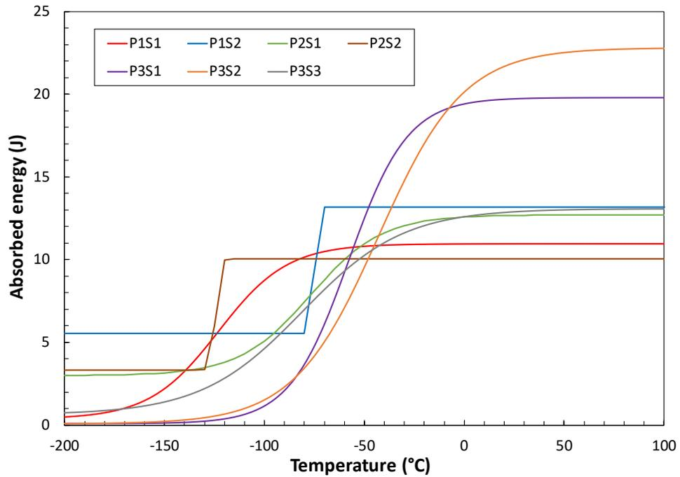
Figure 24 - Absorbed energy transition curves obtained on the base metals of the different pipes and sections in L orientation.
