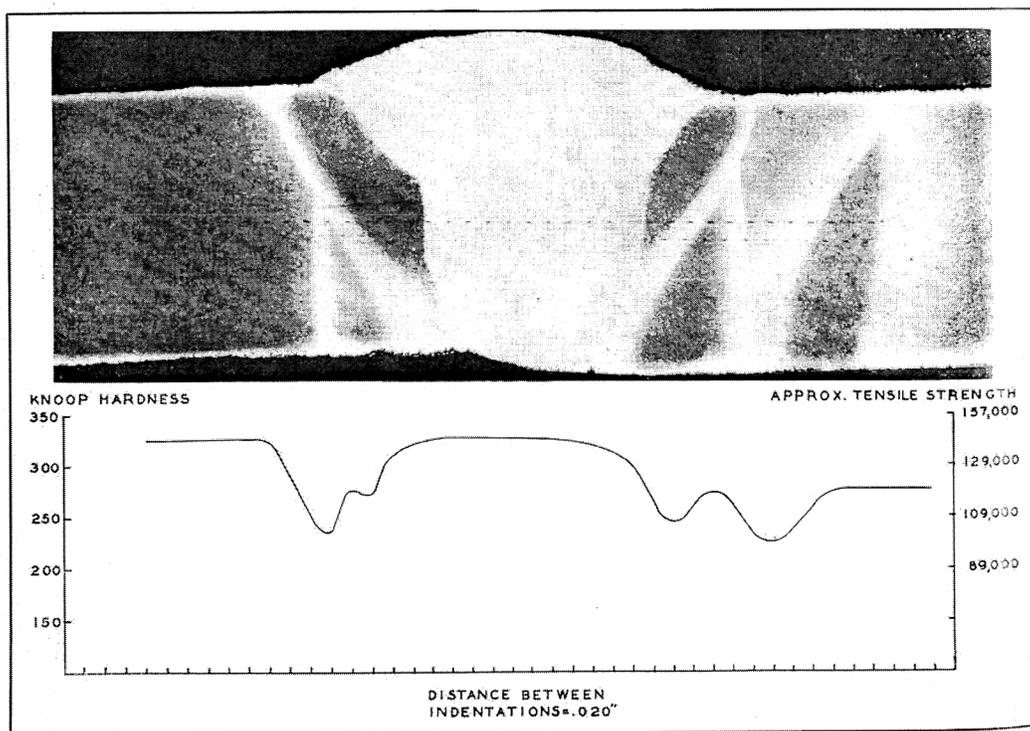
Figure 1 - Knoop indentation trace across a girth weld, from R. S. Ryan (1965).
