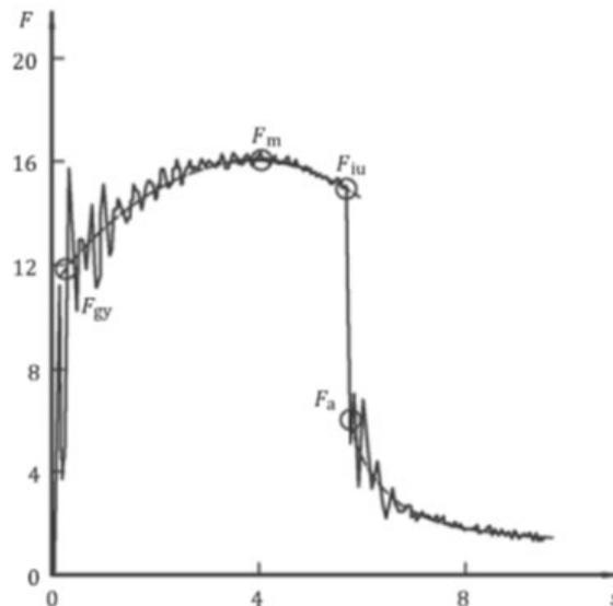
Figure 12 - Example of instrumented force/deflection curve for a test in the ductile-to-brittle transition region.
